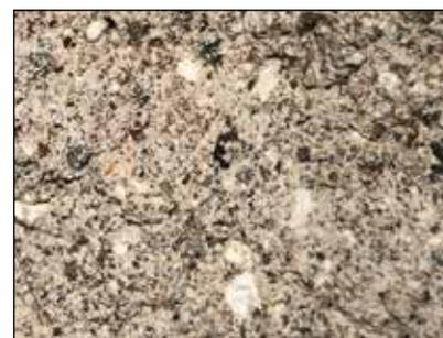
*Lime-rich mortar and render without contraction cracks showing roasted soft lumps of limestone. That on the left is from the late middle ages and on the right from the 18th century. Both with equal parts by weight of lime and whichever aggregate was available.*
