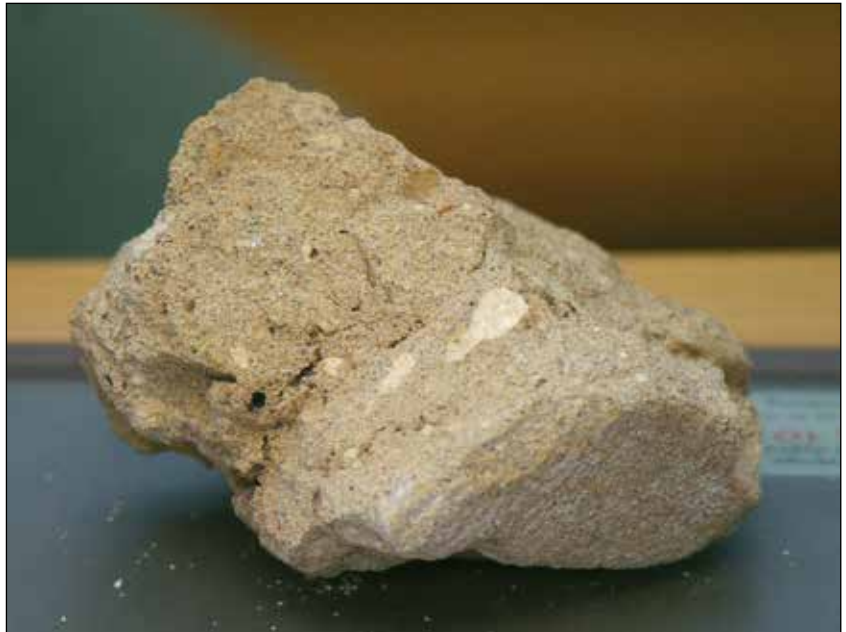
400 year mortar with small lumps of limestone and fragments of charcoal.
