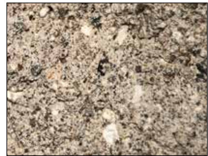
Lime-rich mortar and render without contraction cracks showing roasted soft lumps of limestone. That on the left is from the late middle ages and on the right from the 18th century. Both with equal parts by weight of lime and whichever aggregate was available.
